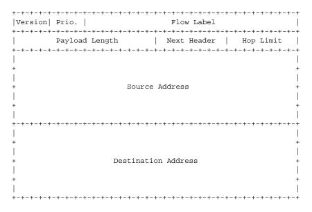
Figure 2: IPv6 Header Format
